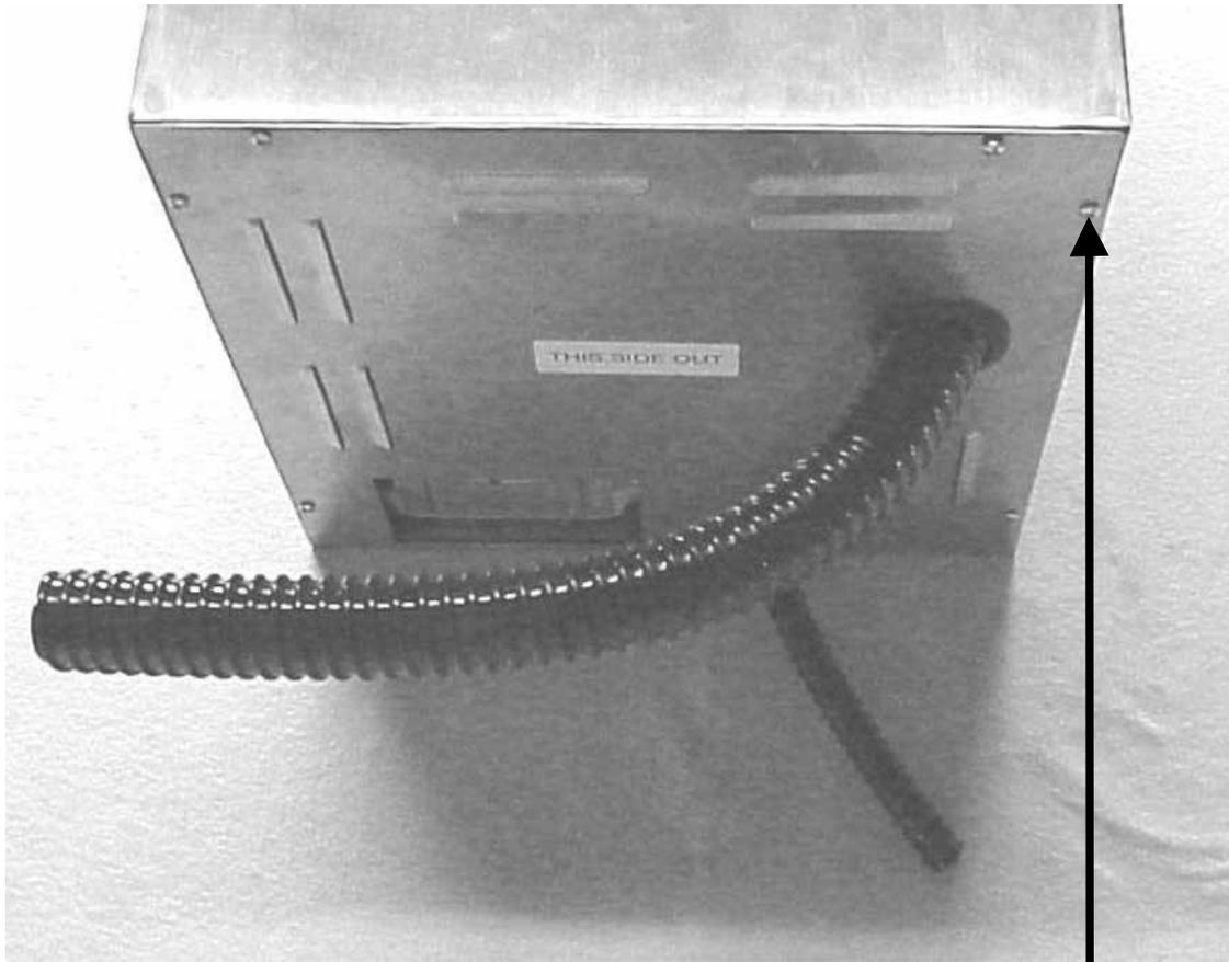
Remove and replace the (2) Plugs with the appropriate Grommets and route the cable or electrical conduit and the factory supplied Drain Hose through their appropriate Grommets prior to fastening the Bottom Plate.
