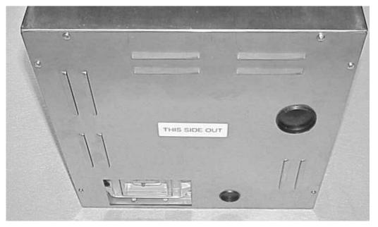
The louvers are facing down, the Label reads "This Side Out", and the two Plugs are installed.
